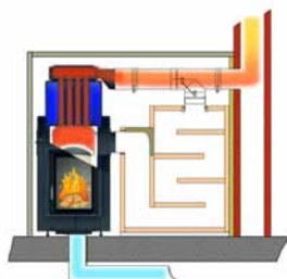
Boiler operation with Moritz's flap
