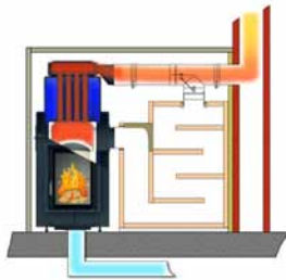
Boiler operation with Moritz's flap
