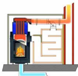
Boiler operation with Moritz's flap
