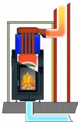
Boiler operation with direct connection
