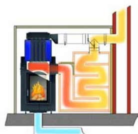
Heat storage mode with Moritz's flap
