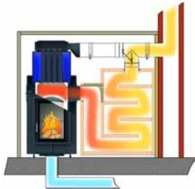
Heat storage mode with Moritz's flap
