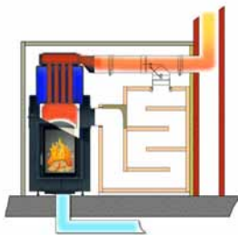
Boiler operation with Moritz's flap
