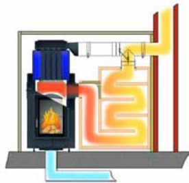
Heat storage mode with Moritz's flap
